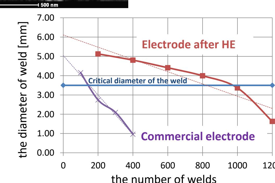
Lifetime of the electrodes treated by HE compared with the lifetime of the reference commercial electrodes [3].
