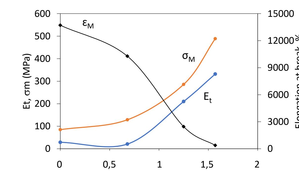
Relationship of mechanical properties determined the tensile test as a function of strain after PA6 HE. Where: tensile modulus ( $E_t$ ), elongation at break ( $\sigma_M$ ), tensile strength ( $\epsilon_M$ ) [2].
