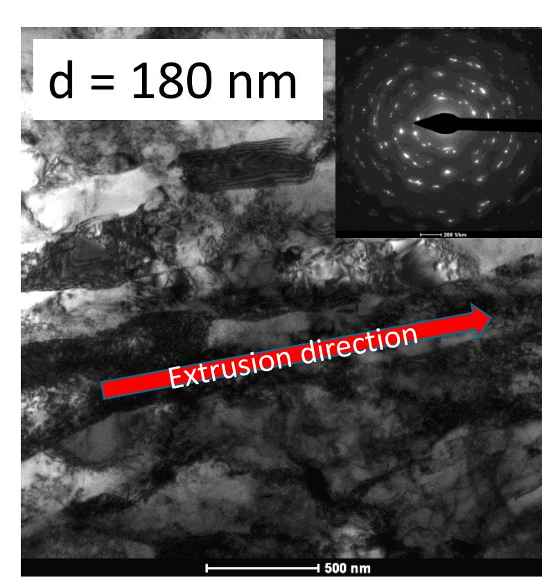
Longitudinal cross-section of CuCrZr ultrafine-grained microstructure after hydrostatic extrusion and artificial aging at 480 °C for 1 h (strong anisotropy).
