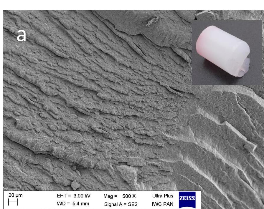
Scanning electron microscopy (SEM) images of cryo-fractured transverse cross-sections of the polyamide PA6 in (a) initial state and (b) rod after cold hydrostatic extrusion HE with true strain  $\epsilon = 1.57$  [2].
