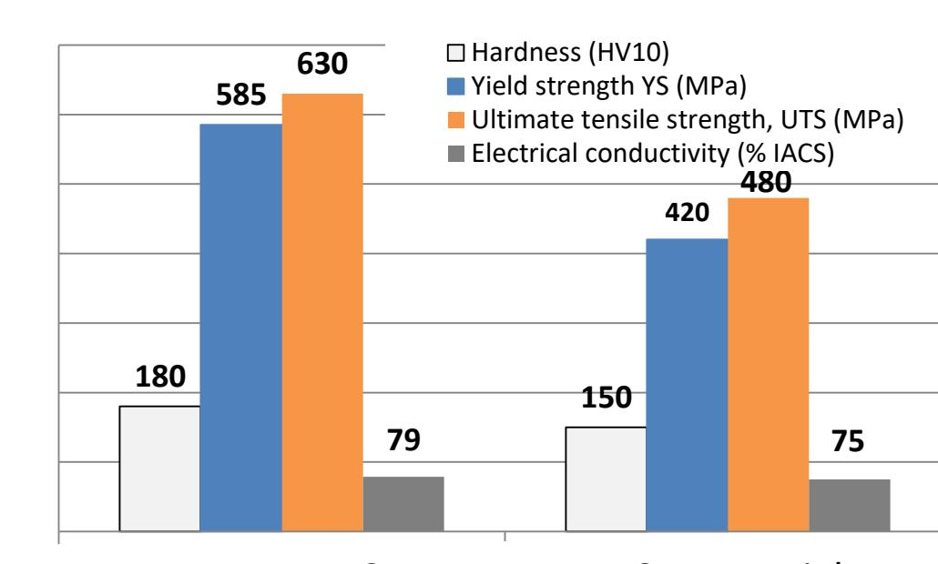
Comparison of hardness, mechanical properties and electrical conductivity between commercial CuCrZr and material after hydrostatic extrusion.
