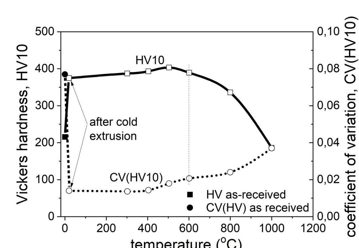
Thermal stability of 316L austenitic stainless steel after cold hydrostatic extrusion [1].
