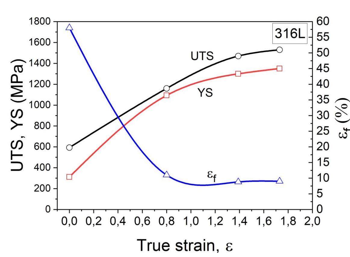
Dependence of the ultimate tensile strength UTS, yield stress YS and elongation to fracture  $\epsilon_f$  on true strain in 316L stainless steel after cold hydrostatic extrusion [1].
